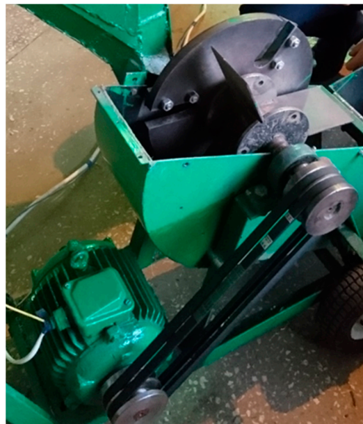
Figure 4. Branch chopper with a disc cutting system.
