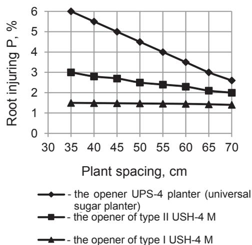
**Figure 2.** The dependence of root injury on the type of the opener.
