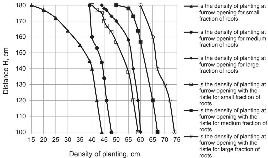
**Figure 6.** The dependence of the density of root planting on the distance between the rear compaction wheels.
