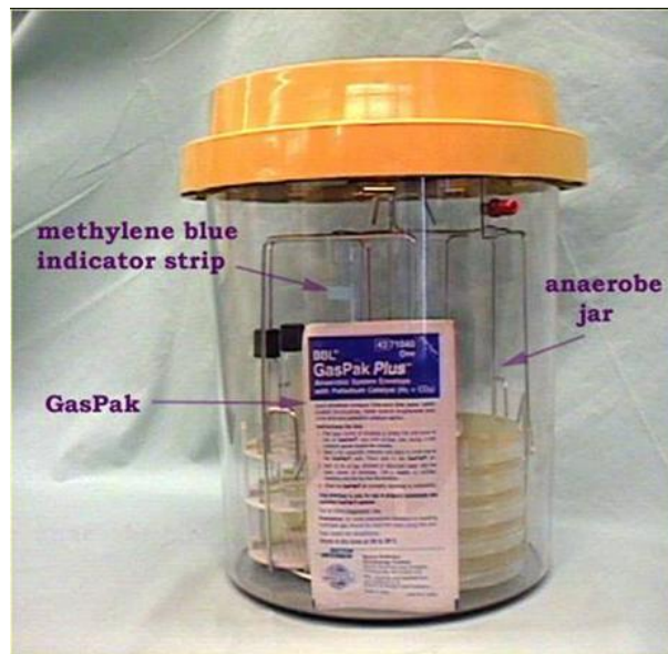
Figure 116. Gas Pak with indicator strip and CO 2 generator pack
