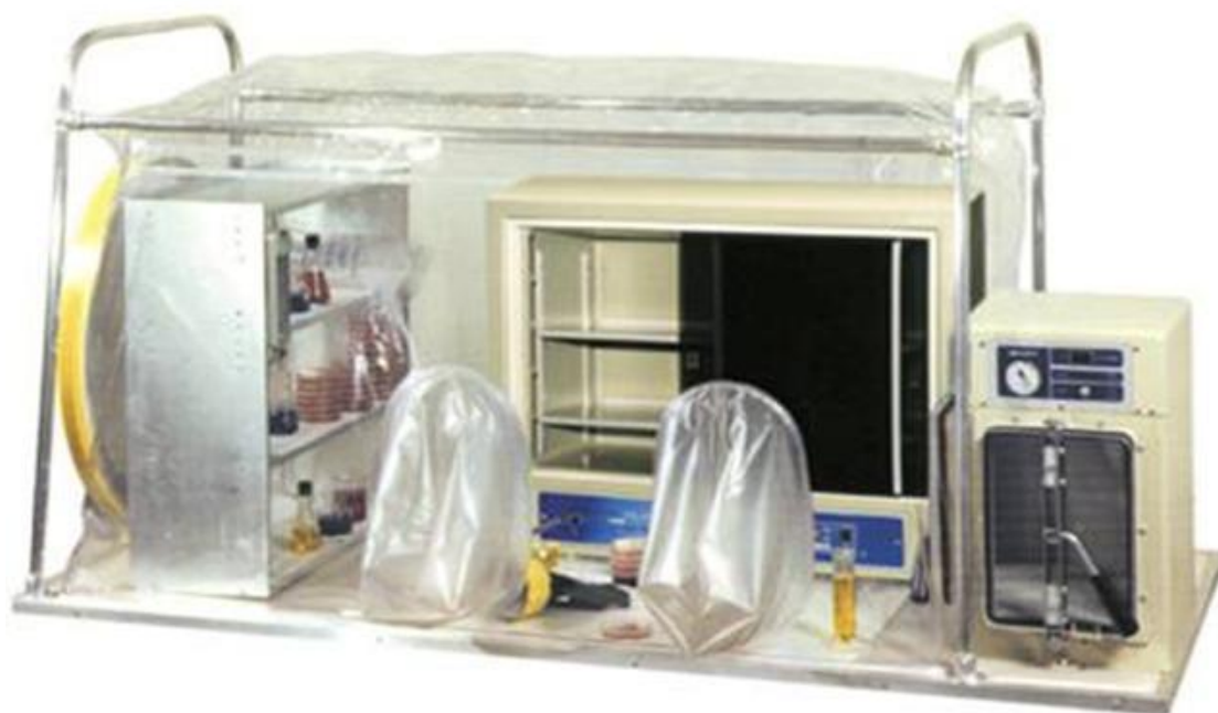
Figure 118. The stationary anaerobic boxes
