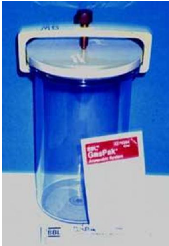
Figure 113. An evacuation and replaceable method foresees the use of anaerobic jar
