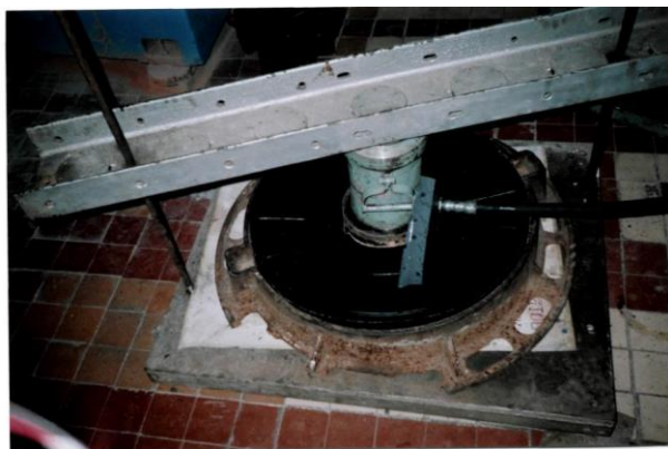
Fig. 6. Testing hatch covers for mechanical strength
