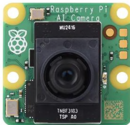
Рисунок 1.2 – Raspberry Pi AI Camera, 12MP, IMX500 Intelligent Vision Sensor
