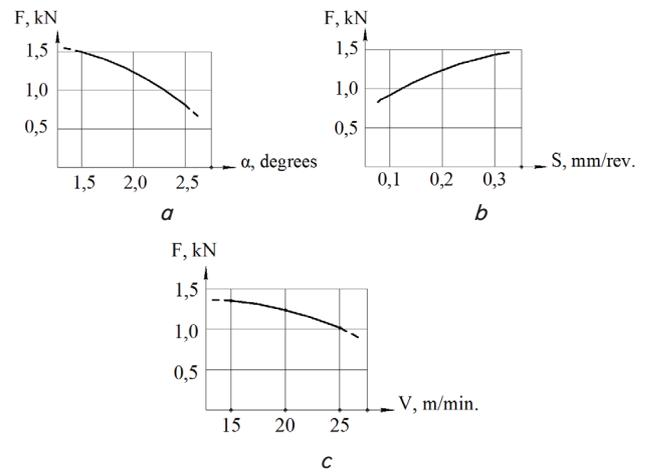
Fig. 6. Dependence of pressing force  $F$ , kN:  $a$  – on the tool entrance angle  $\alpha$ , degrees ( $S=0.2$  mm/rev;  $V=20$  m/min);  $b$  – on the tool supply  $S$ , mm/rev ( $\alpha=2$  degrees;  $V=20$  m/min);  $c$  – on the process rate  $V$ , m/min ( $\alpha=2$  degrees;  $S=0.2$  m/min)
