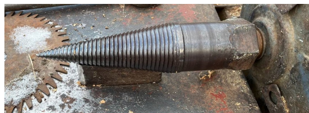
Fig. 1. General view of the active conical deformer (prototype)
