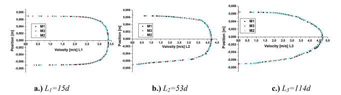
Fig.5. Velocity profiles in the three typical sections for three different densities of the mesh.
