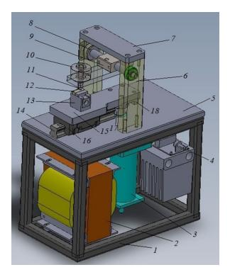
Fig. 1. Constructive model of the test stand СИИП-1 for wear resistance. 1.Frame 2.Transformer 3.Motor-reducer 4.PWM DC controller 5.Main plate 6.Side Beam 7.Connecting beam 8.Axis 9.Loading lever. 10.Load 11.Ball holder 12.Test sample 13.Sample holder 14.Linear guideway 15.Reciprocatingly moving base 16.Ball slider 17.Eccentric 18. Bearing slider
