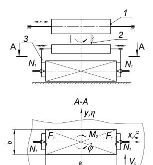
**Figure 5.** The orientation mechanism with captures: 1- the carriage for horizontal relocation of the mechanism of orientation; 2- the drive of a turn of elements of capture with a load; 3- capture element
