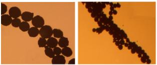
**Figure 5**. Fragments laying ferromagnetic beads: left represented cubic stacking balls not under the influence of the rotational magnetic field, right tetrahedral, under the influence of the rotational magnetic field (microscope ERGAWALL200fold, Germany).
