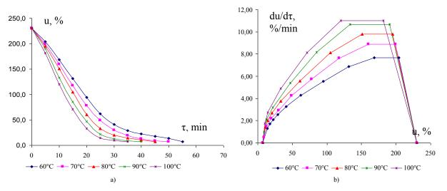
**Figure 3.** Drying curve (a) and drying speed curve (b) of dandelion root by combined method in oscillation regime of 15s /10s
