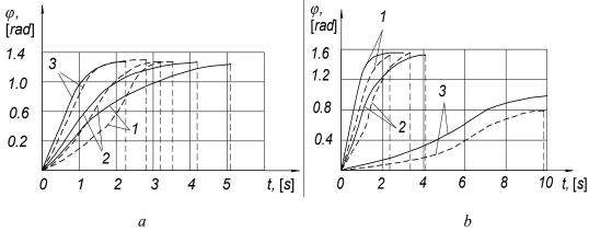
**Figure 2.** Diagrams of change of angular coordinate of a load in the course of its turn an immovable emphasis:
