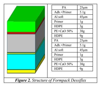
Polyethylene sealing layer is multi-layer to: improve the ability of forming, allow better storage, avoid direct contact of the product with the layer that contains the color of a pigments and a drying part and to arrange a high-power adhesion.
