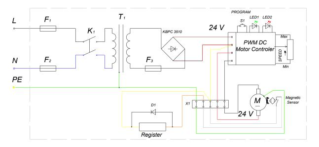
**Fig.2**. *Electric diagram of the test stand СИИП-1 for wear resistance.*
