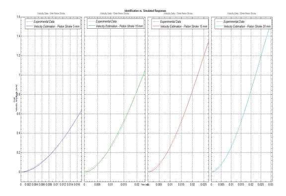
Fig.9 Results of identification of velocity for different strokes of the actuator.
