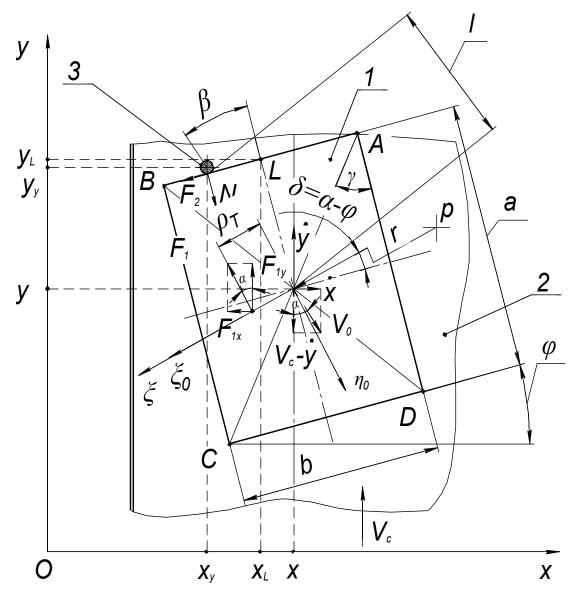
**Figure 1.** The diagram of interaction of forces in case of a turn of a tare load an immovable emphasis on the bearing plane of a packet creating machines : 1- tare load; 2- the bearing plane of the conveyor; 3- fixed bearing
