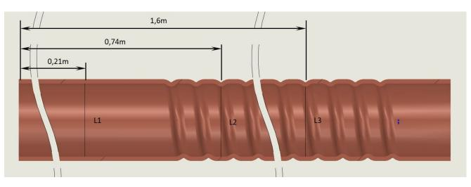
Fig.4. Locations of the created cross sections along the pipeline.
