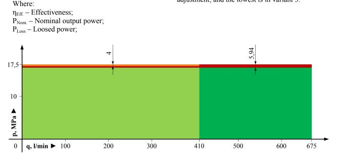
Fig.7 Hydraulic losses, Variant 3
