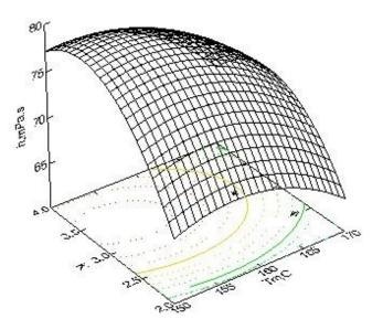
**Fig.3**. Dynamic viscosity  $(\eta, mPa.s)$  depending on moisture content (W, %) and barrel temperature (*Tm*, °*C*) at metering zone temperature 160°C, screw speed 180 rpm, and screw compression ratio 3:1
