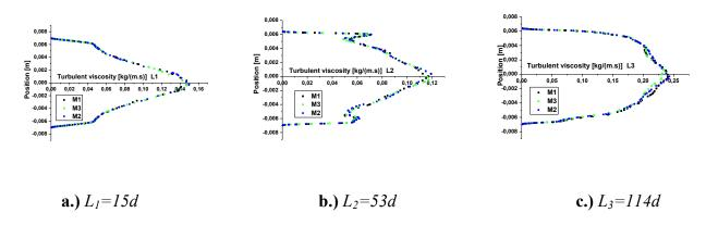
Fig.9. Variation of turbulent viscosity for three different densities of the mesh.
