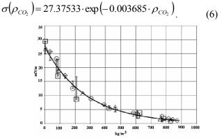
**Figure 4:** Dependence of an interphase tension of oil in contact to CO<sub>2</sub> as function of density dioxide of carbon.
