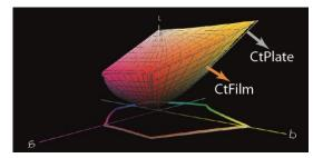
Figure 5. 3D presentation of color gamuts in dependence of plate making technology in CIE Lab, 320% TAC, GCR3 (graph is generated by Chromix Color ThinkPro)
