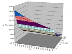
**Figure 3:** Dependence of viscosity of a solution of carbon dioxide in oil from pressure and temperature.
