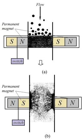
**Figure 3**. Position of permanent magnets: operation N-S (a) and the cleaning process (reverse) S-S (b)
