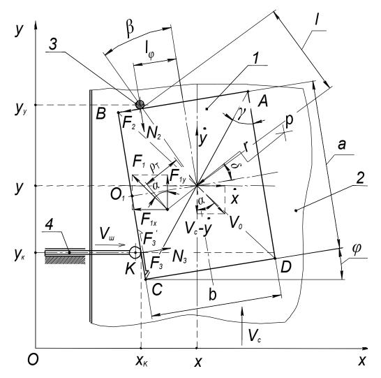
**Figure 3.** The diagram of interaction of forces in case of a turn of a tare load an immovable emphasis on the bearing plane of the conveyor a packet of the creating machine in simul taheus action of a pusher: 1- tare load; 2- the bearing plane of the pipeline, 3- fixed support, 4- pusher
