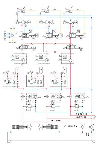
Fig.3 Hydraulic system circuit – Variant 2
