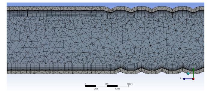
**Fig.3.** *Distribution of the mesh along the pipeline.*
