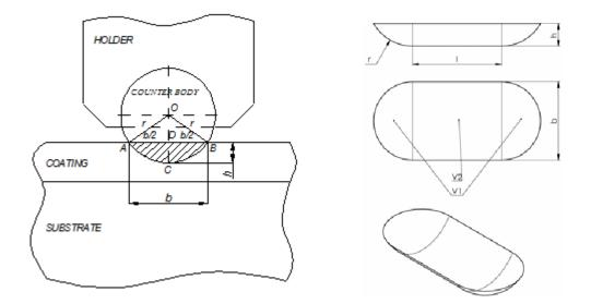
Fig. 4. Chanel on the surface of the test sample in tribological test "ball-on-plate".
