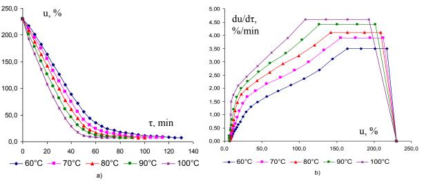
Figure 2. Drying curve (a) and drying speed curve (b) of dandelion root by convective method
