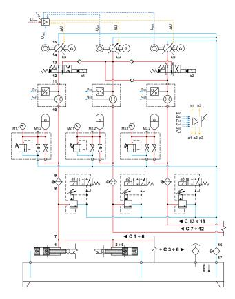
**Fig.2** *Hydraulic system circuit – Variant 1*
