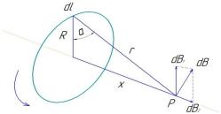
Figure 6. A ring of radius R carrying a current i
