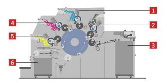
Figure 1. Heidelberg QM DI-46, sheet-fed digital offset printing machine (1-exposure system, 2-offset roller, 3- paper system, 4- plate cylinder, 5-inks system, 6-output device)
