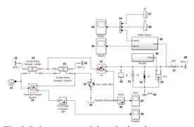
Fig.3 Subsystem modeling hydraulic actuator device and measuring equipment.
