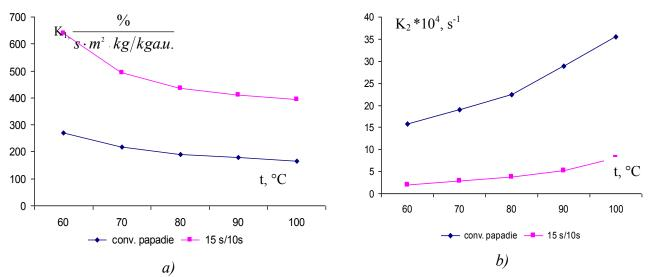
**Figure 4.** *The influence of drying agent temperature on drying speed constants during the first period (a) and the second period (b) for combined and convective drying.*
