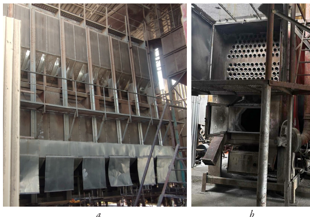
Fig. 3. General view of the elements of the grain dryer: a – Saphir 2134 grain drier; b – biofuel boiler for forming the coolant [14]
