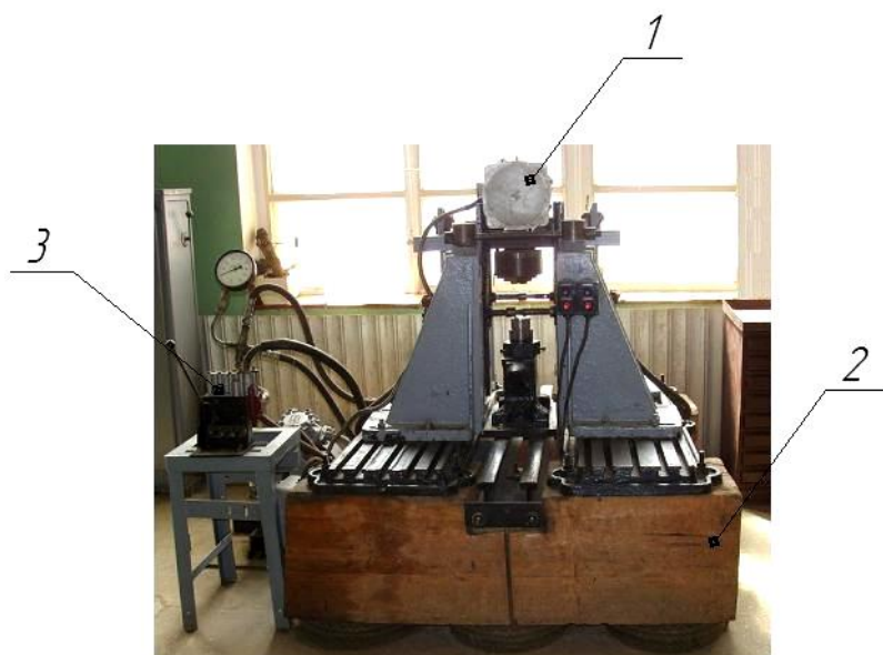
Fig. 3. The general view of vibration installation: 1 – a vibration exciter; 2 – a base; 3 – a hydraulic lifting system
