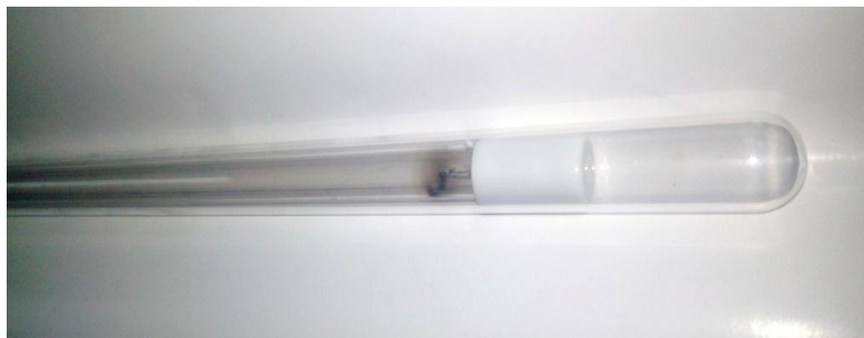
Figure 7.1. Electrical device with a power of 20 W in a quartz case
