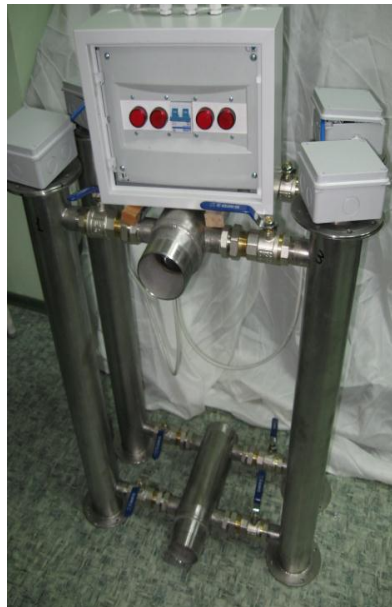
Figure 7.9. Experimental sample of an electrical drinking water disinfection system with a capacity of up to 20 m 3 /h.
