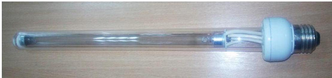
Figure 7.11 Developed electrical device with a power of 15 W (OBIS-15 irradiator)
